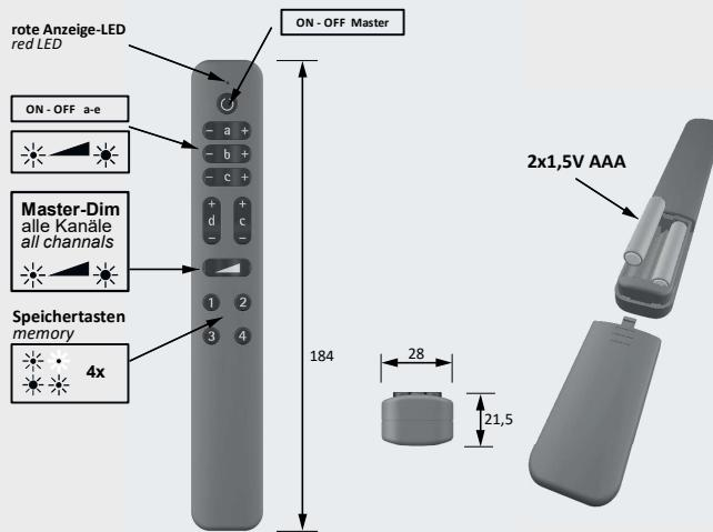
31.101.01 / 31.103.01 Smart Empfänger 4-Kanal smart receiver 4-channel 12VDC/24VDC
